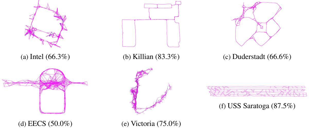
Figure 2.10 Example graphs after CLT sparse GLC node removal. New GLC factors are shown in magenta. The percentage indicates the percentage of nodes that have been removed.
