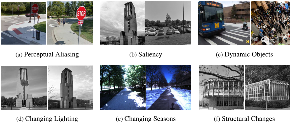
Figure 1.5 Data association challenges. In short-term SLAM applications, the front-end must overcome several challenges including perceptual aliasing, varying measurement saliency and short-term dynamic objects like people and cars. Long-term SLAM is further complicated by longer-term dynamics like lighting, changing seasons, and even structural changes caused by construction. All of these examples occur in the North Campus dataset (Appendix A).
