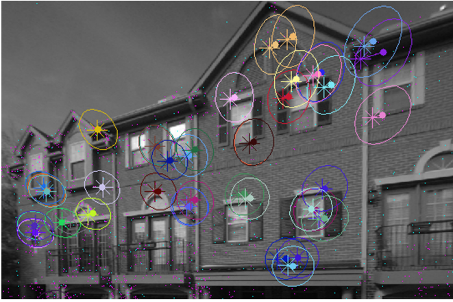
Fig. 5. Geometrically constrained correspondence search. Projected map points are shown as stars and image features are shown as dots. The ellipse around each map feature represents a 99% confidence bound on where the feature should lie in the image.
